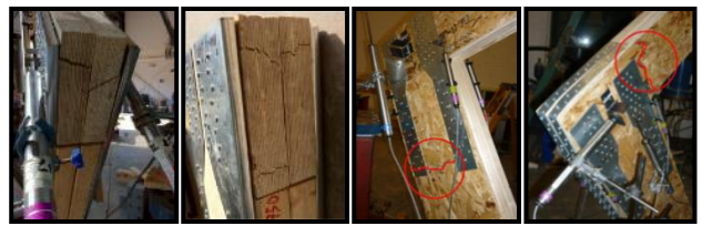
Figure 4: Mode of failure of joints
