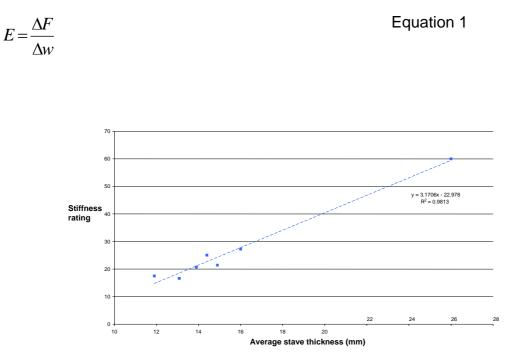
Figure 4 – Stiffness rating comparison of thinned barrels
