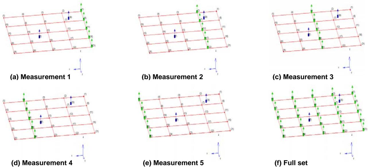
Figure 2: Arrangement of vibration sensors on the metal web joist floor
