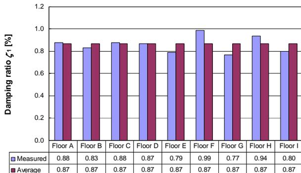
**Figure 5:** Measured damping ratios of metal web joist floors for Mode 1-1
