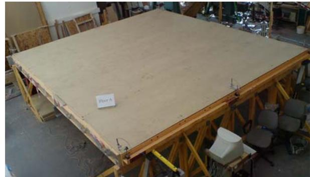
**Figure 1:** A typical metal web joist floor (Floor A)
