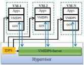
Fig.1. Architecture of VMIDPS for Virtualized Environment
