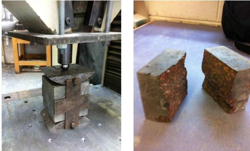
**Figure 5-5** Splitting tensile testing
