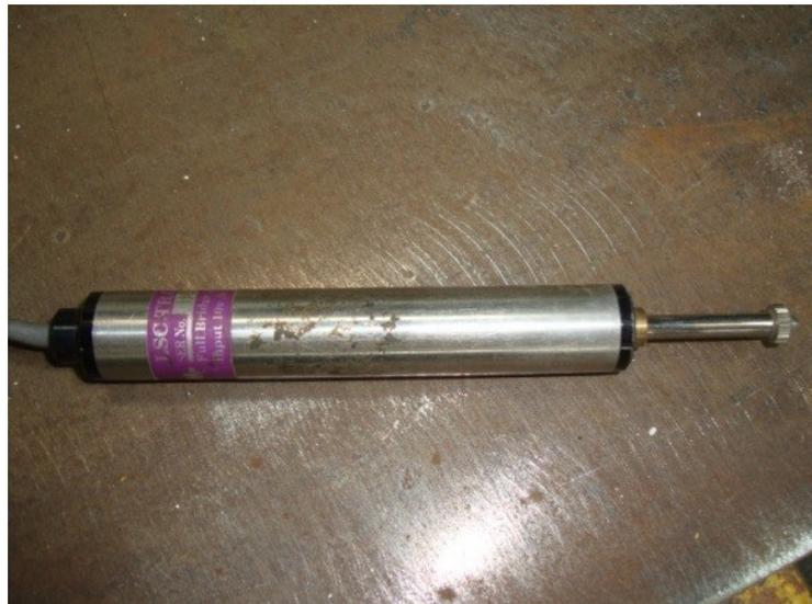
**Figure 5-9** The linear variable differential transducer (LVDT)
