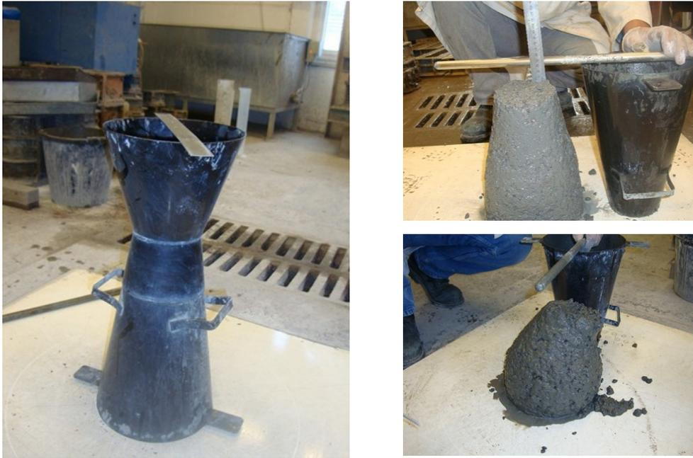
**Figure 5-1** Slump testing
