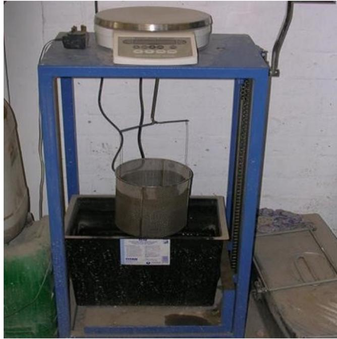
**Figure 5-7** Density testing apparatus (weight-in-air/weight-in-water method)
