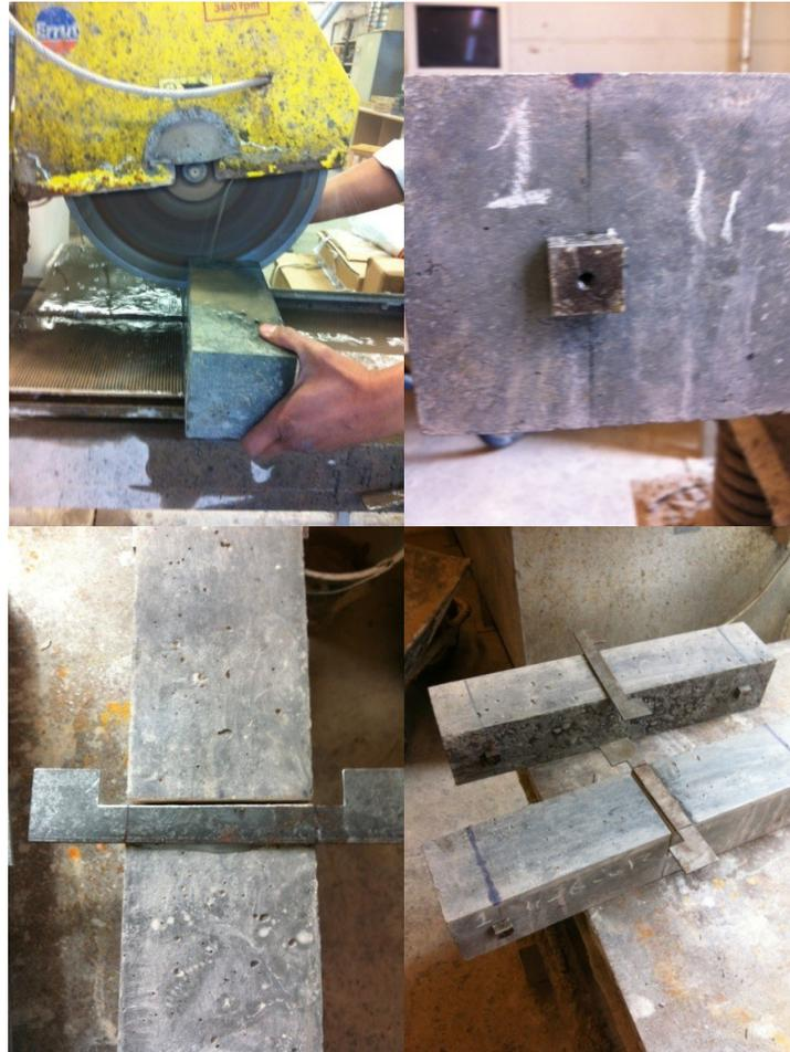
**Figure 4-4** Beam samples with notches at mid-span
