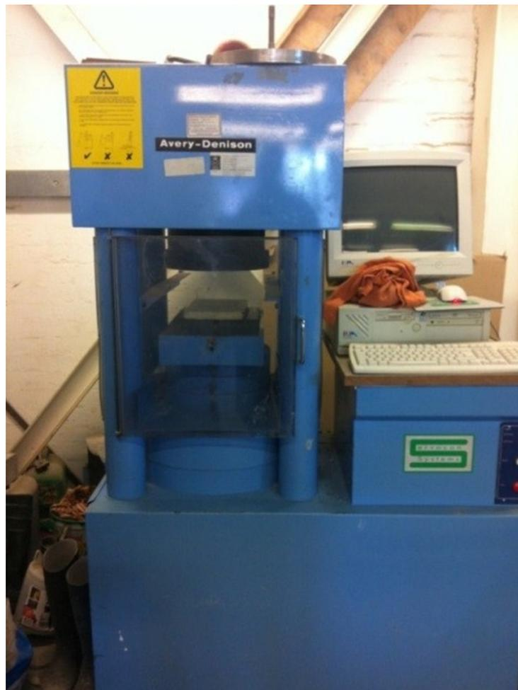
**Figure 5-2** The 3000 kN Avery Denison testing machine
