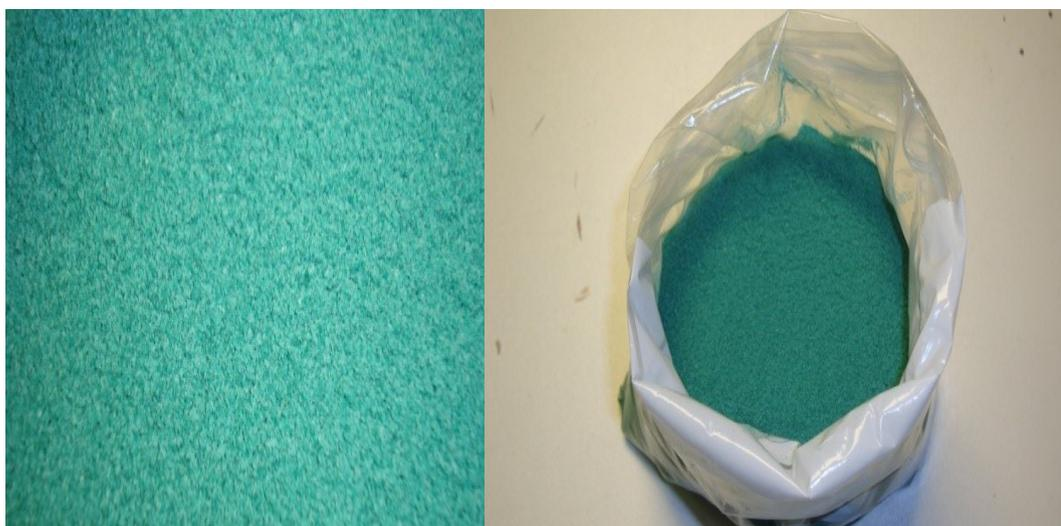
**Figure 3-9** The LLDPE powder used in this study
