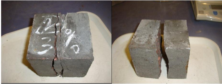
**Figure 6-15** Failure patterns of the HPC specimens under splitting tension
