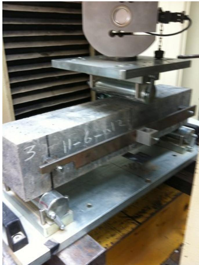
**Figure 5-11** Three-point bending test set-up
