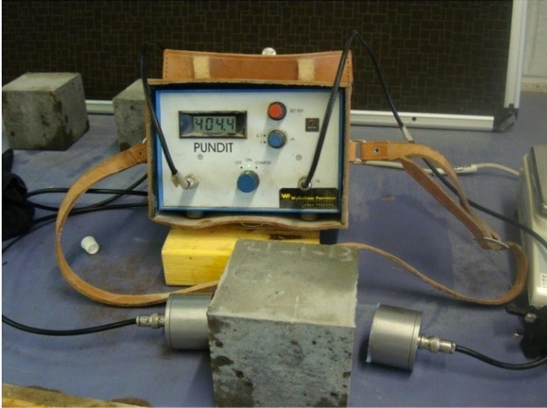
**Figure 5-6** Pundit ultrasonic tester for measuring the dynamic elastic modulus
