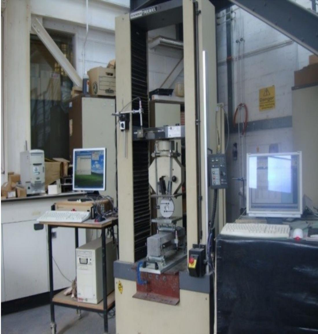
**Figure 5-8** Fracture toughness testing in the 5500 R Instron testing machine
