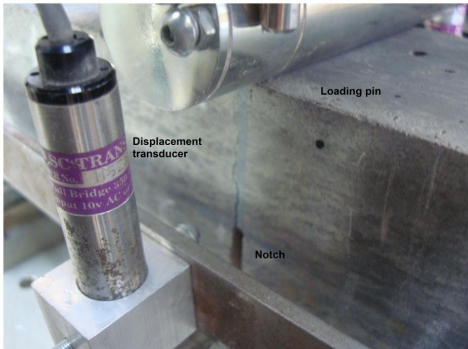
**Figure 5-12** A notched beam during three-point bending testing
