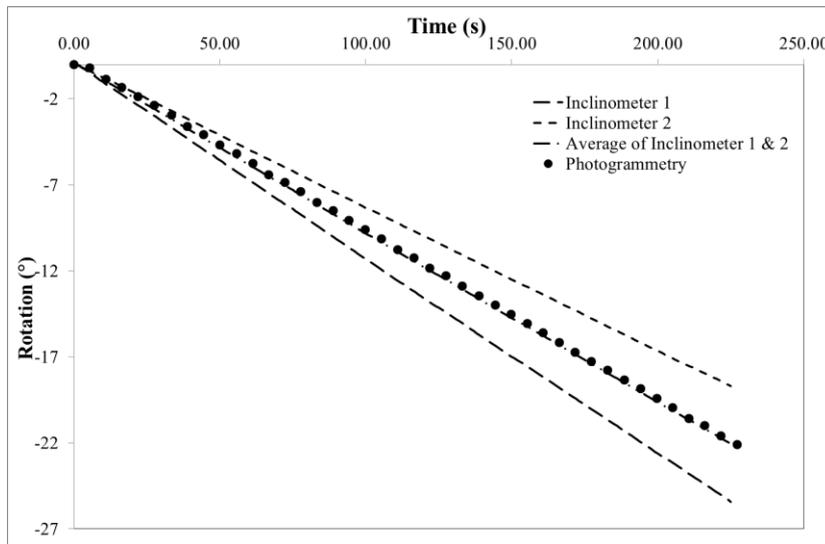
Figure 4 Comparison of the inclinometer and photogrammetric measurement for Sample 1
