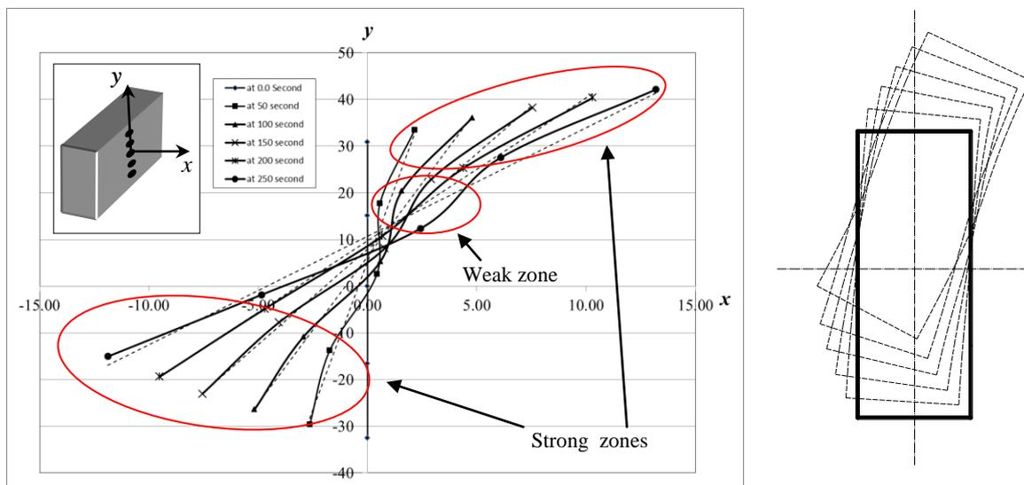
Figure 6 (a) Displacement of longer side of the cross-section (b) Original and deformed cross-section
