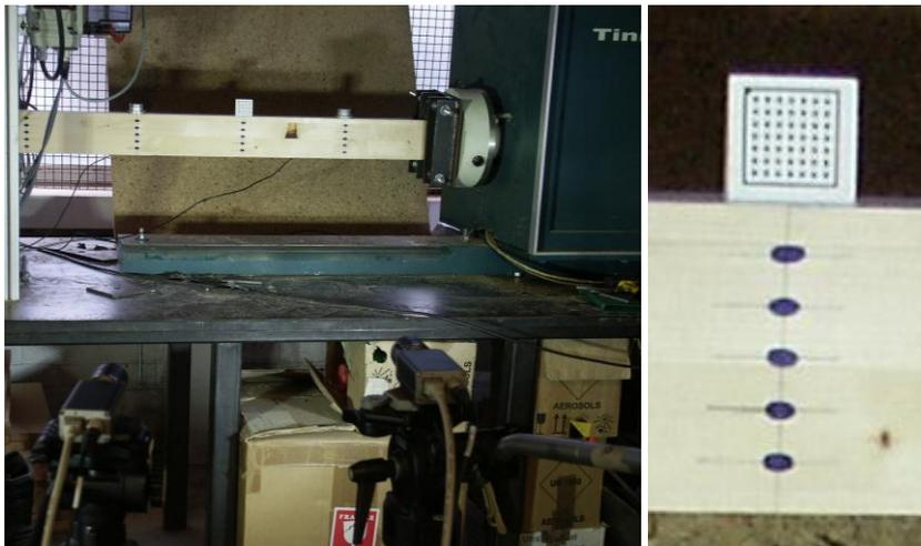
Figure 1. Experiment setup, location of calibration plate and target points
