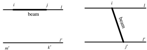
Figure 4: Two Arrangements of Beam Elements in a Strip
