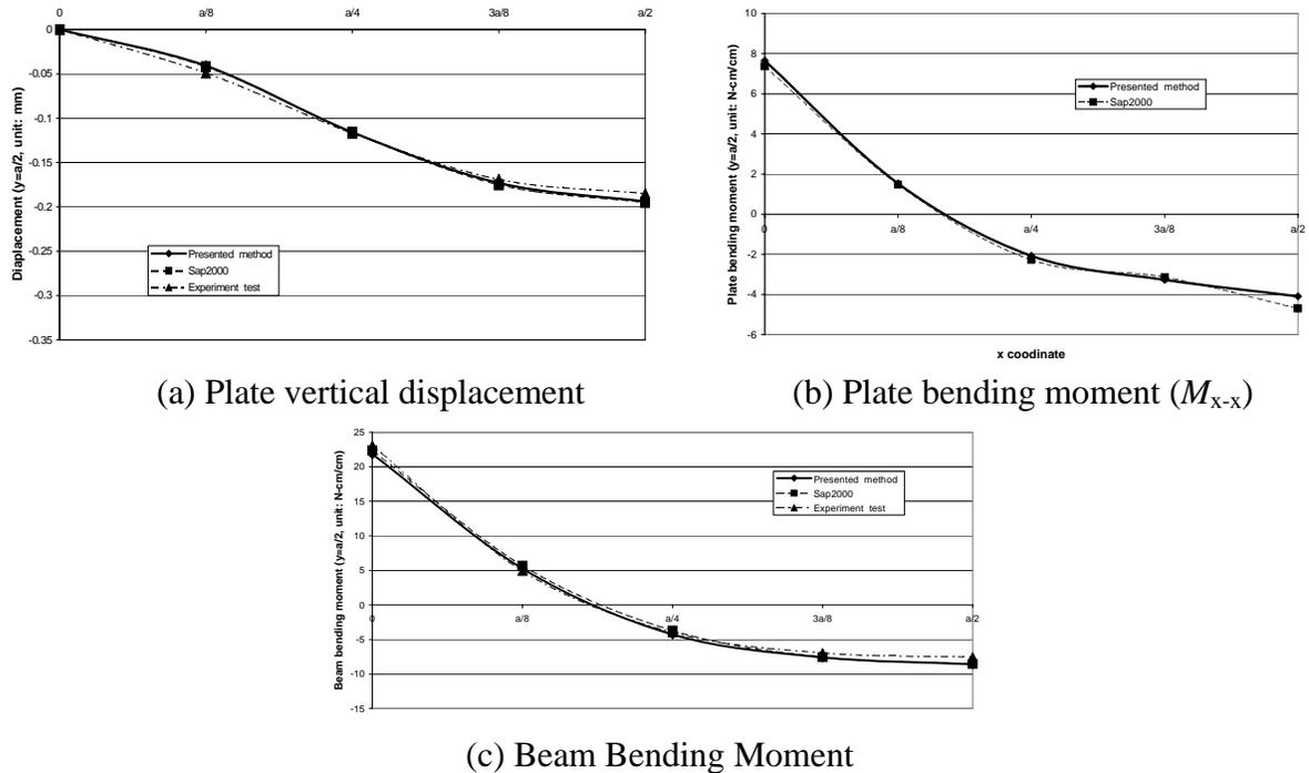
Figure 8: Displacements and Bending Moments of Plate Stiffened by Two Orthogonal Beams along Symmetrical Axis  $y = a/2$
