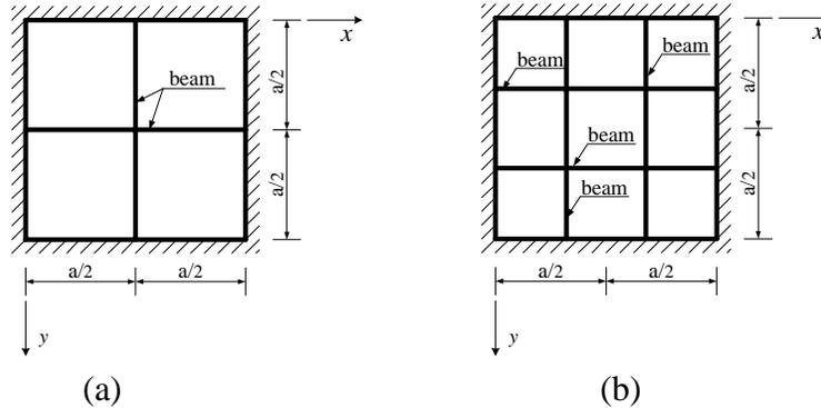
Figure 7: Square Stiffened Plates with Fixed edges ( $a = 20.18$  cm). (a) Stiffened by Two Orthogonal Beams; (b) Stiffened by Four Orthogonal Beams
