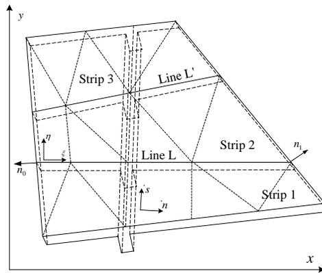
Figure 1: Analogous Stiffened Plate for General Plate-and-Grid Structures
