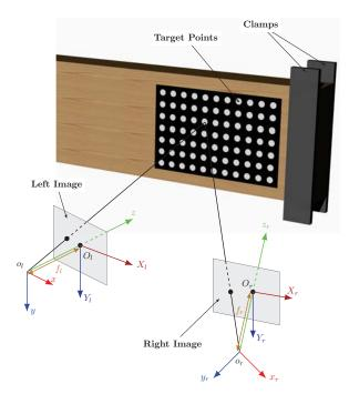
Fig. 1 Target points reconstruction of binocular stereo vision
