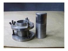
Figure 7. Reinforced crushing pot designed by Lőrincz, used for crushing tests. (A Lőrincz által tervezett mini-mozsár)
