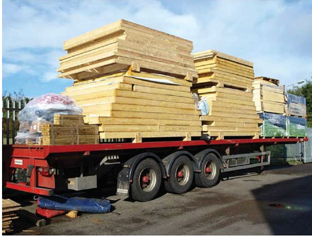
Fig. 5. Examples of different transport methods for offsite timber panels and a volumetric module, whose height necessitates the use of an articulated trailer: (a) Standard trailer with stacked open timber panels; and (b) Articulated trailer with a volumetric timber module. Photograph(s) taken by: Duncheva, T.
