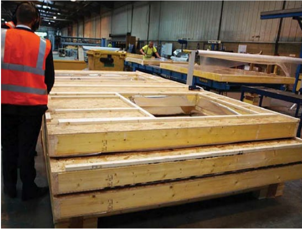
Fig. 1. Examples of offsite timber systems studied in this paper: (a) Closed timber panels; and (b) Volumetric timber module. Photograph(s) taken by: Duncheva, T.
