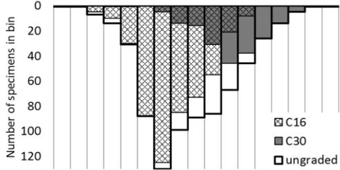
Figure 1: Distributions of (a) bending strength, (b) bending stiffness and (c) density for UK larch graded to C16/C27/reject and C16/C30/reject with a Brookhuis mtgBATCH 962 (total of 706 specimens)
