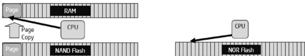
Figure 17 Access pattern of NAND and NOR memories (credit: FIORILLO, 2009)
