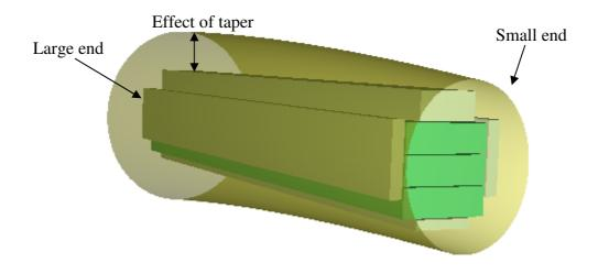
Figure 2.1. Example cutting pattern in highly tapered log.
