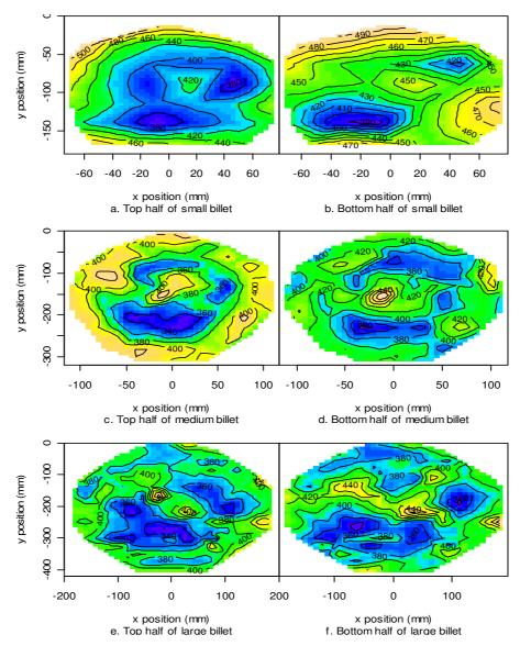
Figure 5.9. Density distributions (at 12% MC) within the top and bottoms half of each test billet. a and b, small billet. c and d, medium billet. e and f, large billet. Units of the contours are in kg  $m^{-3}$ .
