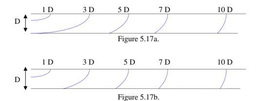
Figure 5.17. Model of wave shape using an elliptical rather than a spherical propagation shape. a. Value obtained from Bucur and Berndt (2001): longitudinal velocity 3 times faster than tangential. b. Value obtained from Zhang et al. (2011): longitudinal velocity 2.5 times greater than radial.
