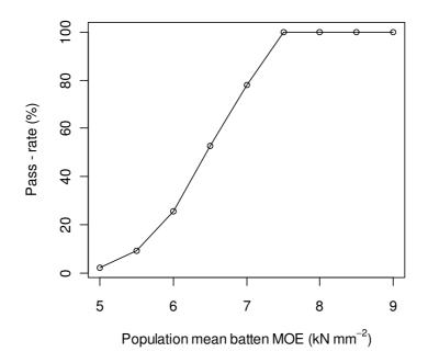
Figure 6.14. C16 pass-rate of battens with falling population mean MOE.
