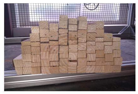
Figure 5.5. Strips reassembled to their correct positions within the test billet.
