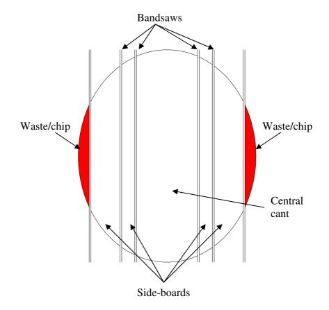
Figure 6.5. Log primary breakdown system.
