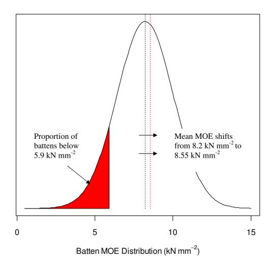
*Figure 6.2. Illustration of how removal of all battens below 5.9 kN mm*<sup>-2</sup> *results in the mean batten MOE shifting from 8.2 kN mm*<sup>-2</sup> *to 8.55 kN mm*<sup>-2</sup>.
