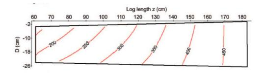
Figure 5.18. From Zhang et al. (2011). Small log stress wave contour maps in longitudinal-radial plane of red pine logs. Impacting point: z=0. Contour unit: microseconds ( $\mu$ s).
