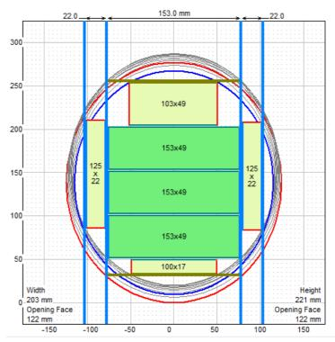
Figure 2.5. Typical sawmill cutting pattern.
