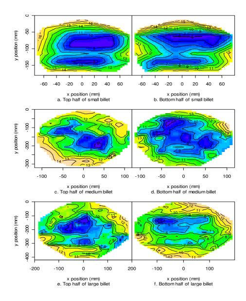
*Figure 5.10. Distribution of dynamic MOE (at 12% MC) within the top and bottoms half of each test billet. a and b, small billet. c and d, medium billet. e and f, large billet. Units of the contours are in kN mm*<sup>-2</sup>.
