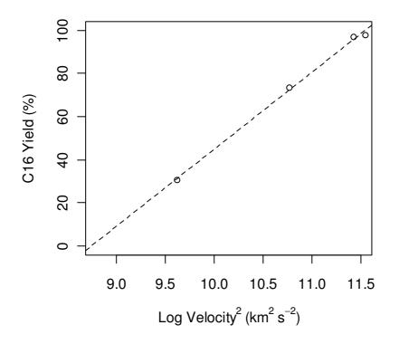
*Figure 6.13. Relationship between log velocity<sup>2</sup> and C16 yield.*
