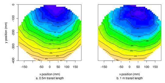
Figure 5.14. TOF contour graphs for the large billet for the a) 0.5 m transit length and b) 1.0 m transit length. The units for the contour lines are in microseconds.
