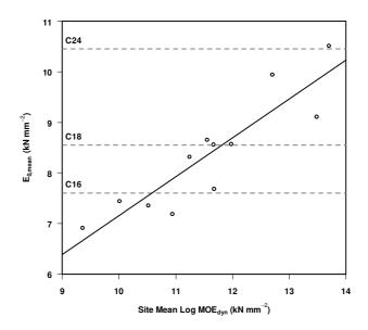
*Figure 6.1. From Moore et al. (in press). Mean timber bending stiffness versus mean log dynamic stiffness for 12 sites around Scotland and northern England.*
