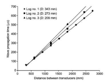
*Figure 5.19. From Zhang et al. (2011). Relationship between wave propagation time and distance between two transducers.*
