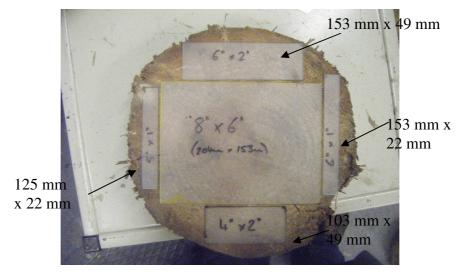
*Figure 6.4. Example cutting pattern being transcribed onto a disc.*
