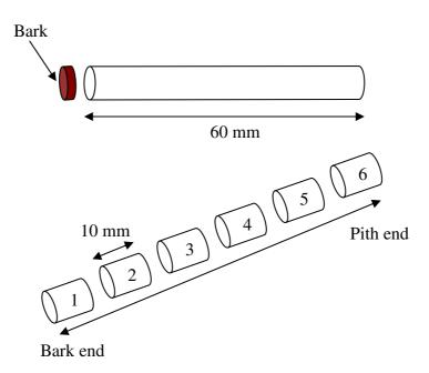
Figure 4.1. 60 mm long increment core before and after being broken up into 10 mm lengths for density measurement.
