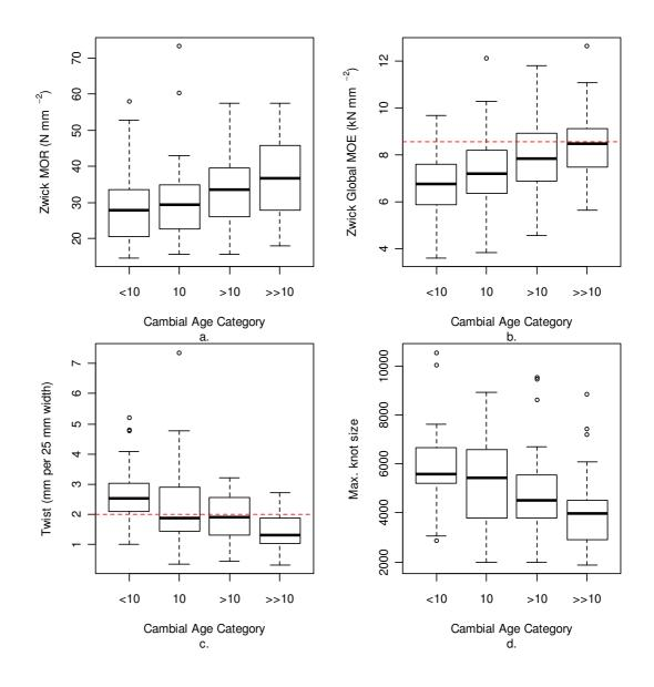
Figure 6.12. The effect of cambial age on (a) MOR, (b) Global MOE. The dotted line represents the average MOE required for C18. (c) Twist (at 12% MC). The dotted line represents the visual override grade limit for strength classes C18 and below. (d) Overall knot severity.
