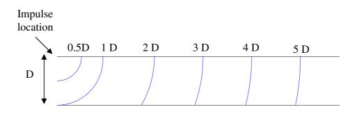
*Figure 5.16. Spherical propagation of wavefront in a cylinder.*
