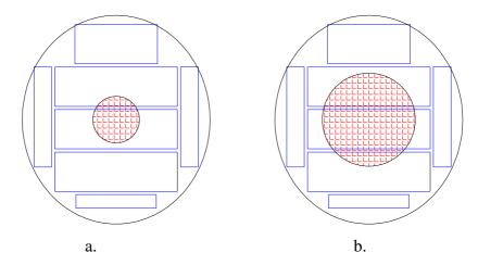
Figure 2.6. The proportion of juvenile wood in structural battens when JW takes up a) 5% and b) 20% of the cross section.
