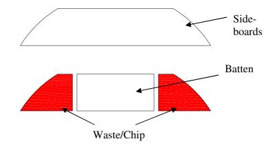
Figure 6.6. Edging system for slabs from primary breakdown.
