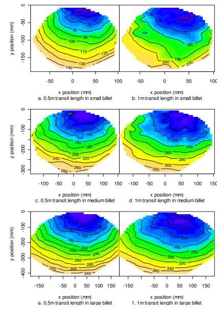
Figure 5.7.Contour graphs of the TOF arrival time for the 0.5 m and 1.0 m transit lengths. a and b, small billet. c. and d, medium billet. e. and f, large billet. The stress wave was initiated at the same azimuth as co-ordinate (0,0). Units of the contours are in microseconds.
