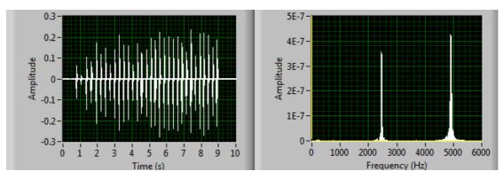
*Figure 5.6. Example of resonant sound recording and its resulting frequency spectrum of a 1.0 m strip.*
