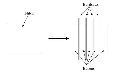
Figure 6.8. Final breakdown of a flitch.
