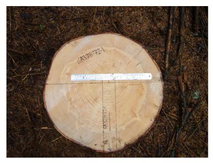
Figure 4.2. Marking of 50 mm wide strip that was extracted from the breast height disc to verify corer density measurements.
