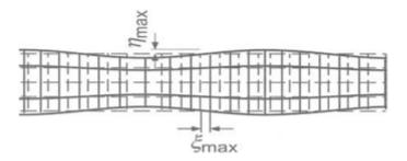
Figure 2.2. The lateral contraction,  $\eta_{max}$ , due to the axial extension,  $\xi_{max}$ , caused by the passing stress wave (from Cremer et al. 2005).
