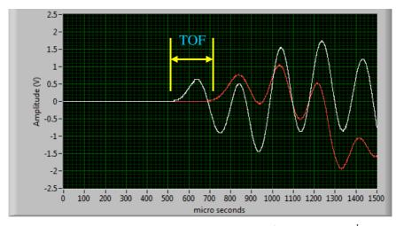
Figure 5.4. An example waveform showing the  $1^{st}$  (grey) and  $2^{nd}$  (red) receiver probe signals over a 1.0 m transit length.
