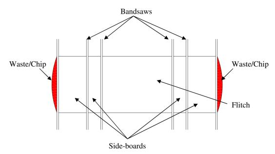
Figure 6.7. Secondary breakdown of the central cant.
