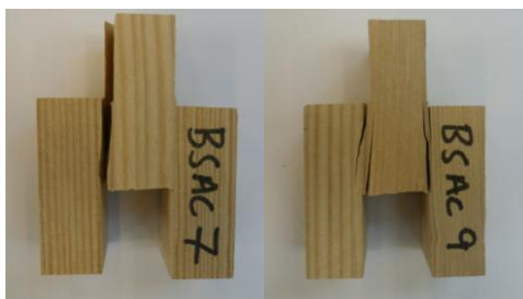
Figure 14: Bond strength failure modes
