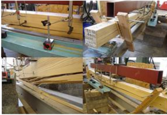
Figure 12: GluLam Failure modes
