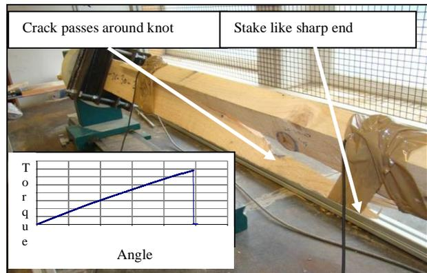
**Figure 7:** A combined shear tension failure occurred in 2.8m joist and crack passed through knot and ends up with a sharp end
