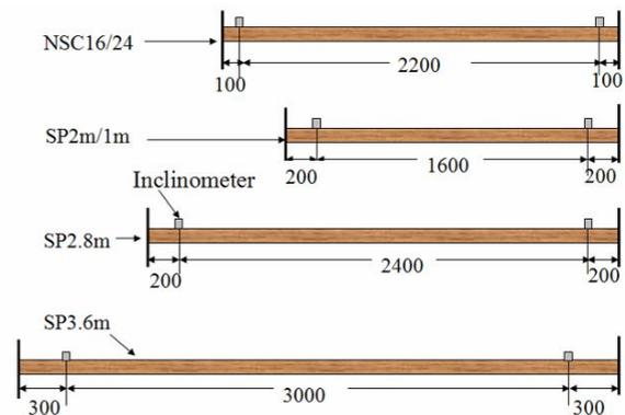
Figure 2: Shear strength test arrangements for SP and NS joists (lengths in mm)
