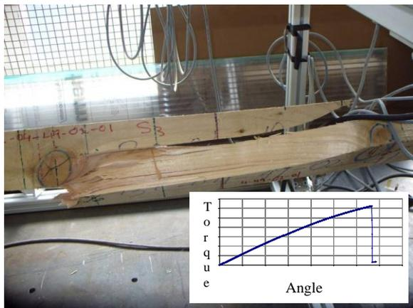
**Figure 7:** A typical shear failure occurred in 2.8m specimen due to top and bottom edge knots
