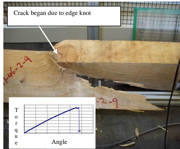
**Figure 8:** A typical shear failure began due to an edge knot in 3.6m joist
