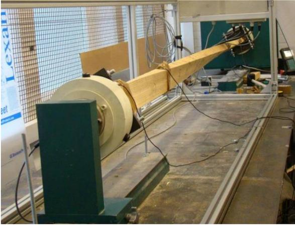
**Figure 4:** A typical 3.6 m joists with large rotational deformation before the fracture
