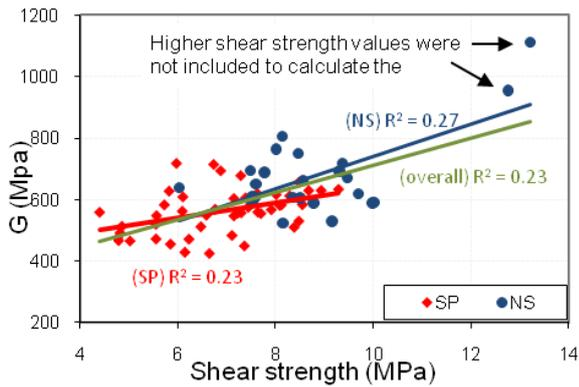
**Figure 12:** Linear relationship between  $G$  and the shear strength of SP and NS joists
