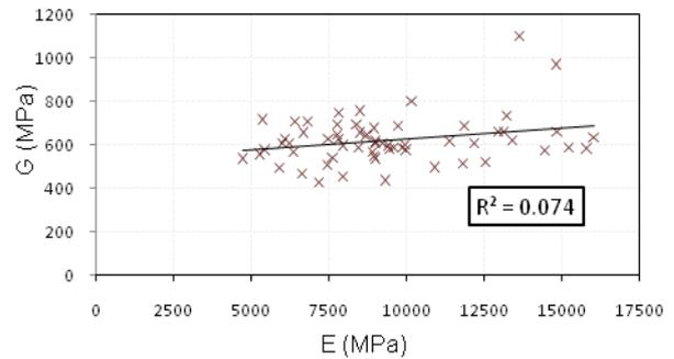
**Figure 15:** Linear relationship between  $G$  and the (dynamic acoustic)  $E$  at span level
