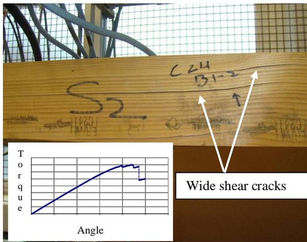
**Figure 11:** A typical wide shear cracks occurred in C24 timber joists under torsion loading
