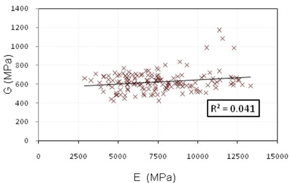
**Figure 14:** Linear relationship between  $G$  and the (global)  $E$  of 1800 mm sections
