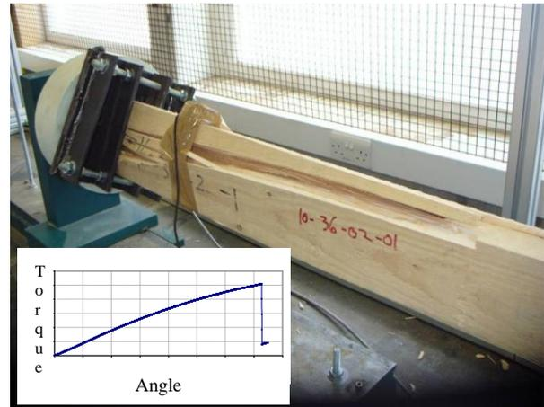
**Figure 6:** A crushing failure of 3.6m batten and its torque-twist relationship
