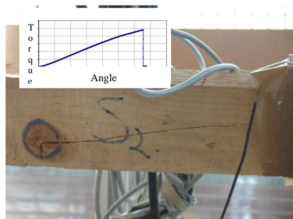
**Figure 9:** A typical shear crack started from knot fissure
