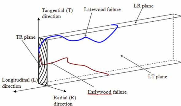
**Figure 5:** Schematic diagram of timber joists showing grain direction
