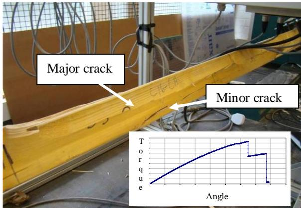
**Figure 10:** A typical NS C16 batten with a large horizontal shear crack and minor cracks
