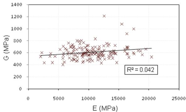
**Figure 13:** Linear relationship between  $G$  and the (local)  $E$  of 600 mm sections
