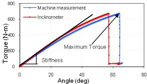
**Figure 3:** A typical applied torque and relative twist of 2.8m test sample
