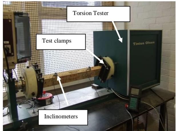
Figure 1: Torsion testing apparatus 1.0 m sample
