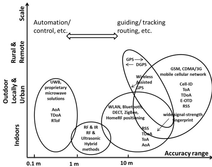
Figure 11- List of various wireless-based positioning systems
