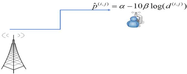
Figure 5. RSS for distance estimation
