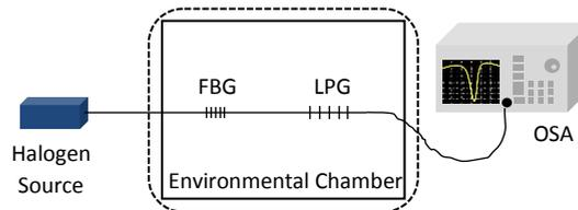
Fig. 2 – Experimental setup for temperature calibration.
