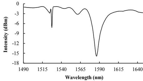
Fig. 1 – The transmission spectra of the FBG/LPG hybrid sensor.
