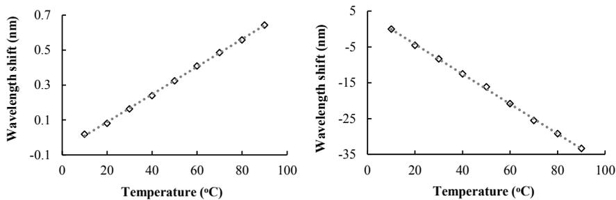
Fig. 3 – Temperature variation on the bare hybrid sensor; FBG (left) and LPG (right) performance.
