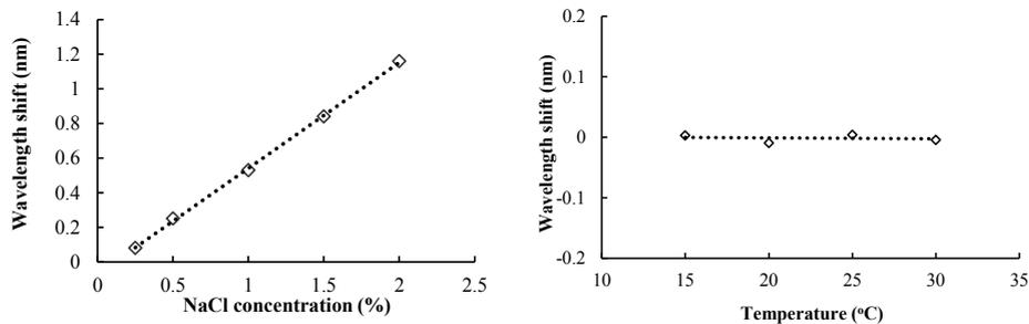
Fig. 4 – Wavelength shift of the LPG due to NaCl concentration variations at  $30^\circ\text{C}$  (left) and temperature compensated LPG wavelength shift due to varying temperature at  $1\% \text{NaCl}$  concentration (right).
