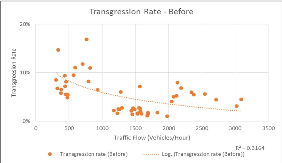
**Figure 5: Transgression Rate by Traffic Flow Before Stud Implementation**
