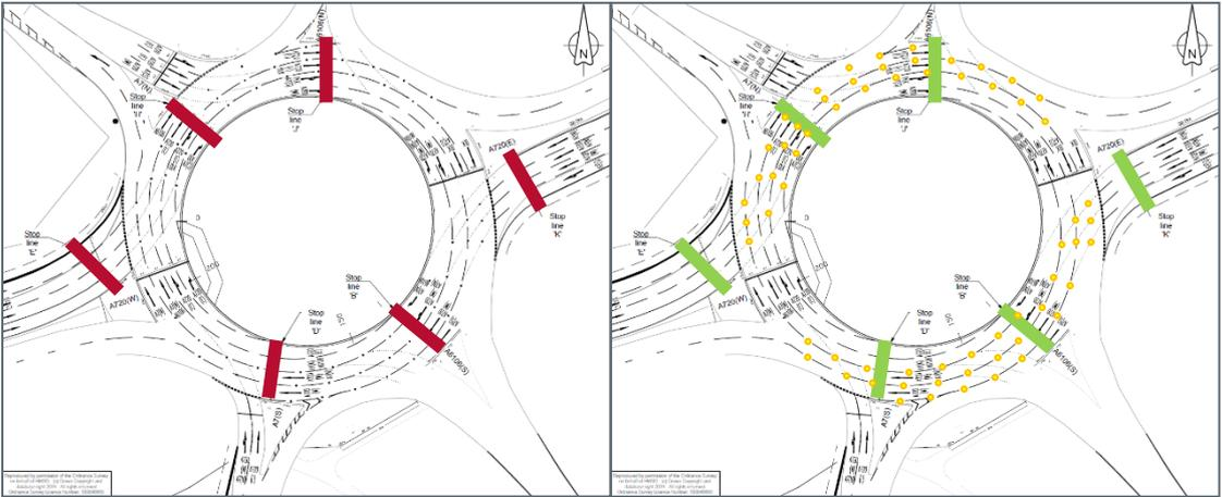
Figure 3: Co-ordination of studs with traffic signals
