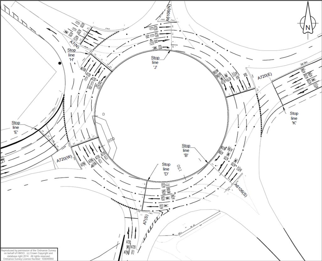
Figure 2: Layout of Intelligent Road Studs (Source: Amey)
