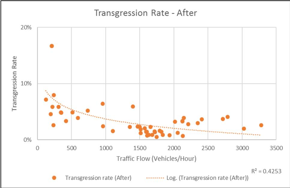
**Figure 6: Transgression Rate by Traffic Flow after Stud Implementation**
