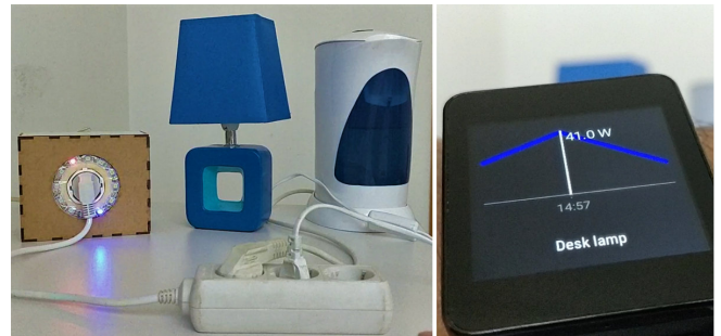
Figure 3. Wattom’s NILM capabilities enables the distinction between various appliances connected simultaneously. Wattom displays a colored target per appliance (left), which upon selection sends the energy consumption of that device to the user’s smart watch (right).
