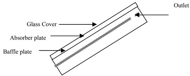
**Figure 4, Schematic diagram of heater by Garg and Rani [9]**
