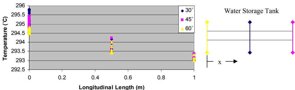
Figure13, Temperatures along the depth of the heater at three segments
