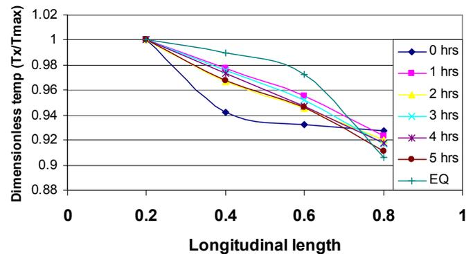
Figure 6, Dimensionless temperatures along the longitudinal length for  $\phi= 45^\circ$ , 100W
