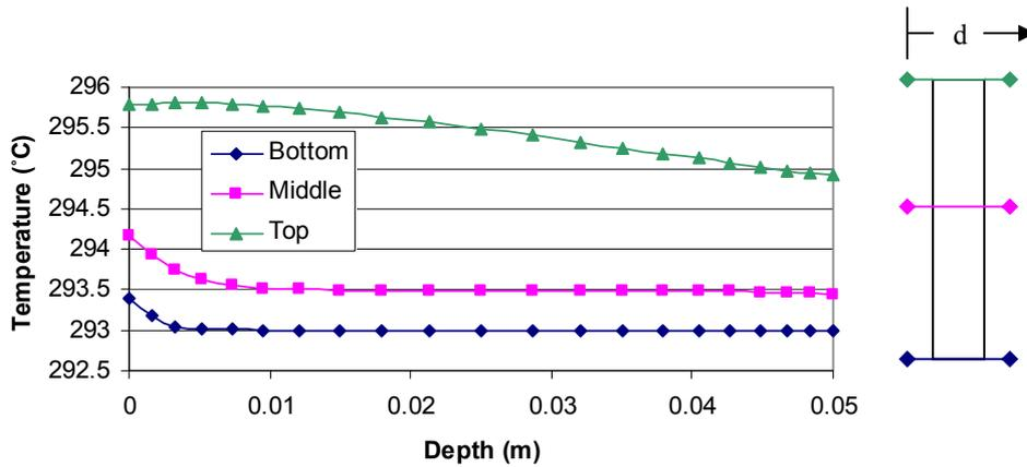
Figure 14, Temperature along the depth of the heater at three segments
