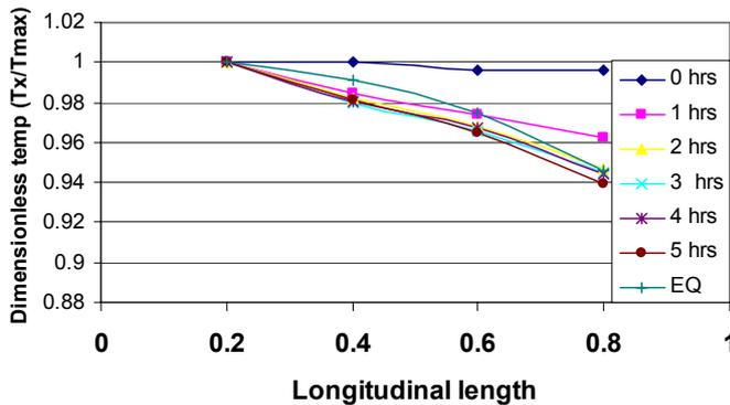
Figure 7, Dimensionless temperatures along the longitudinal length for  $\phi= 60^\circ$ , 100W
