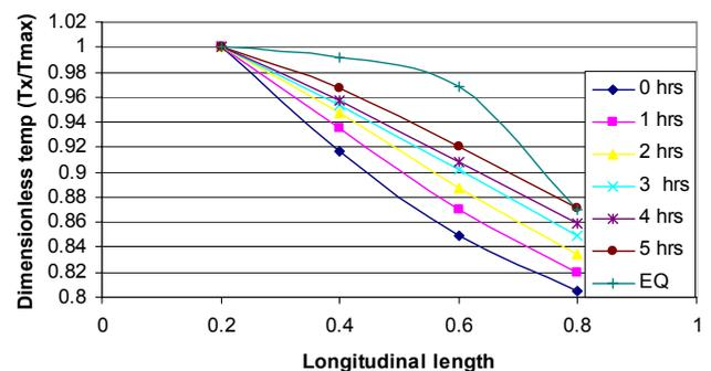
Figure 10, Dimensionless temperatures along the longitudinal length for  $\phi= 60^\circ$ , 200W
