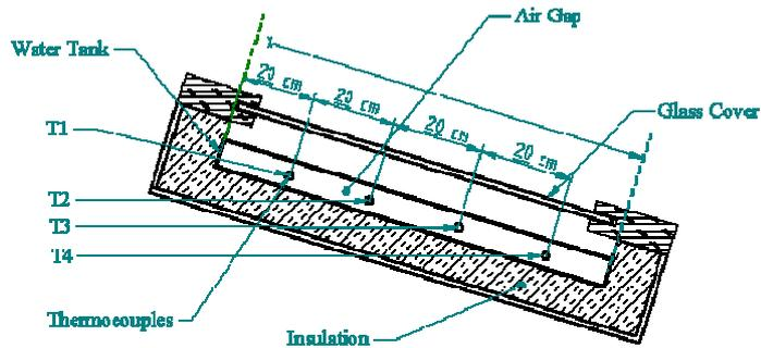
Figure 1, Rectangular storage ICS collector; the location of thermocouples is also shown.
