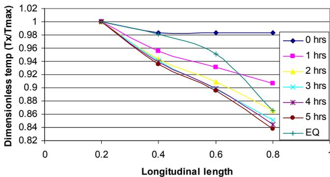
Figure 9, Dimensionless temperatures along the longitudinal length for  $\phi= 45^\circ$ , 200W
