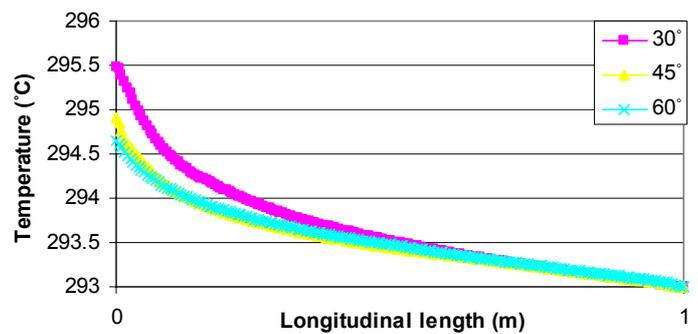
Figure 12, Temperature profile along the longitudinal length at the middle plane through CFD analysis for  $\phi = 30^\circ, 45^\circ$  and  $60^\circ$  after 20 min
