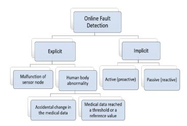
Fig. 7. Fault detection in WBAN
