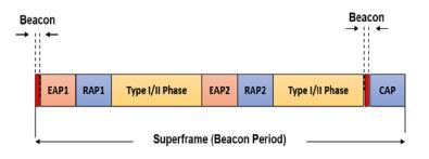
Fig. 3. IEEE802.15.6 beacon mode superframe structure
