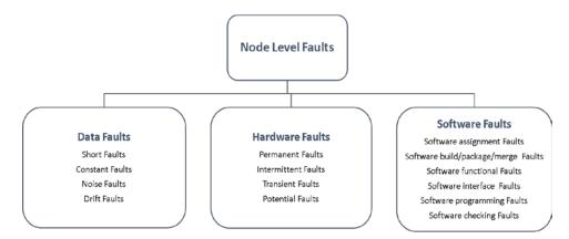
Fig. 4. Faults at node level in wireless communication
